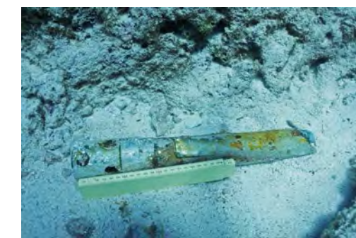
BELOW The .50-caliber gun muzzle with identifying plate helped pinpoint the wreckage as that of a P-40K Warhawk. Photo by Kelly Keogh/NOAA
