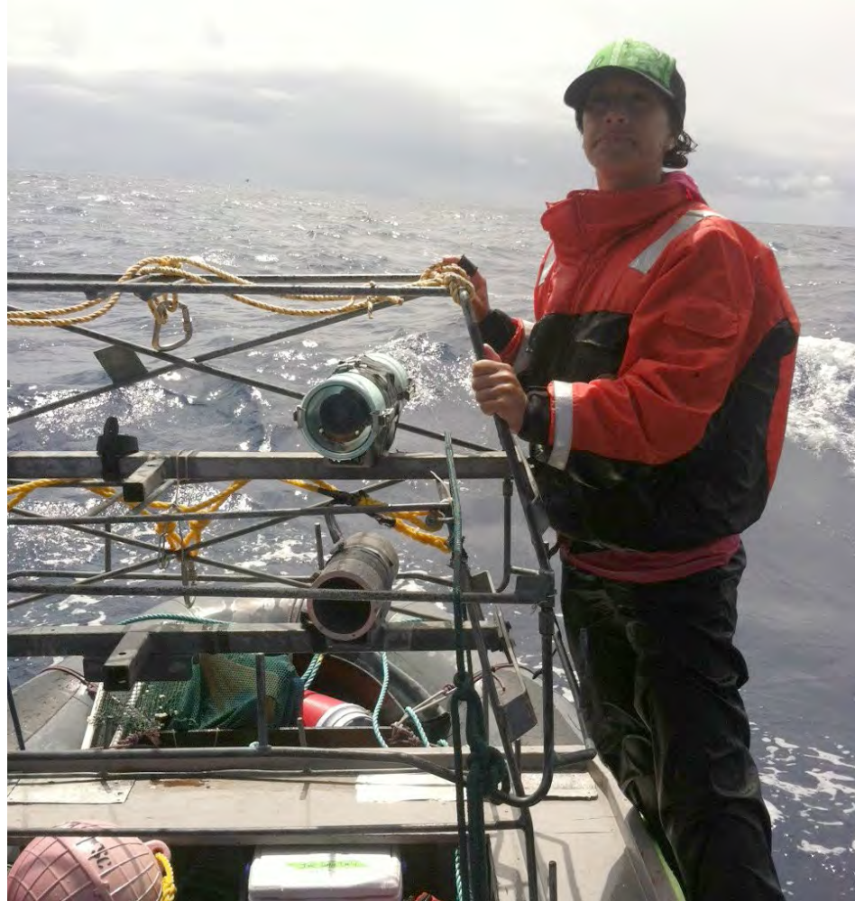
RIGHT Emily Crigler and affiliate prepares to deploy a BRUV. Photo by Jacob Asher/NOAA
