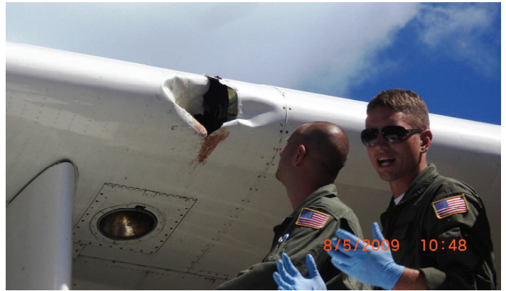
Damage to the wing of USCG C-130 aircraft after an unfortunate collision with a great frigatebird
